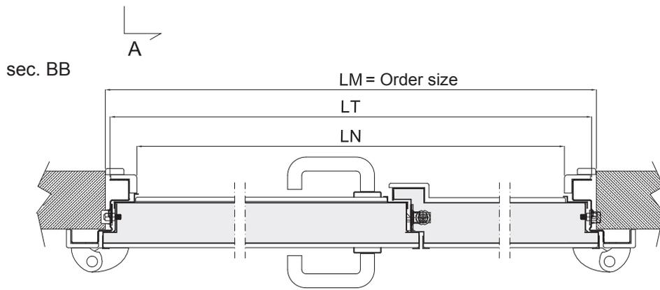
LN (nominal size) variable according to coating thickness.
